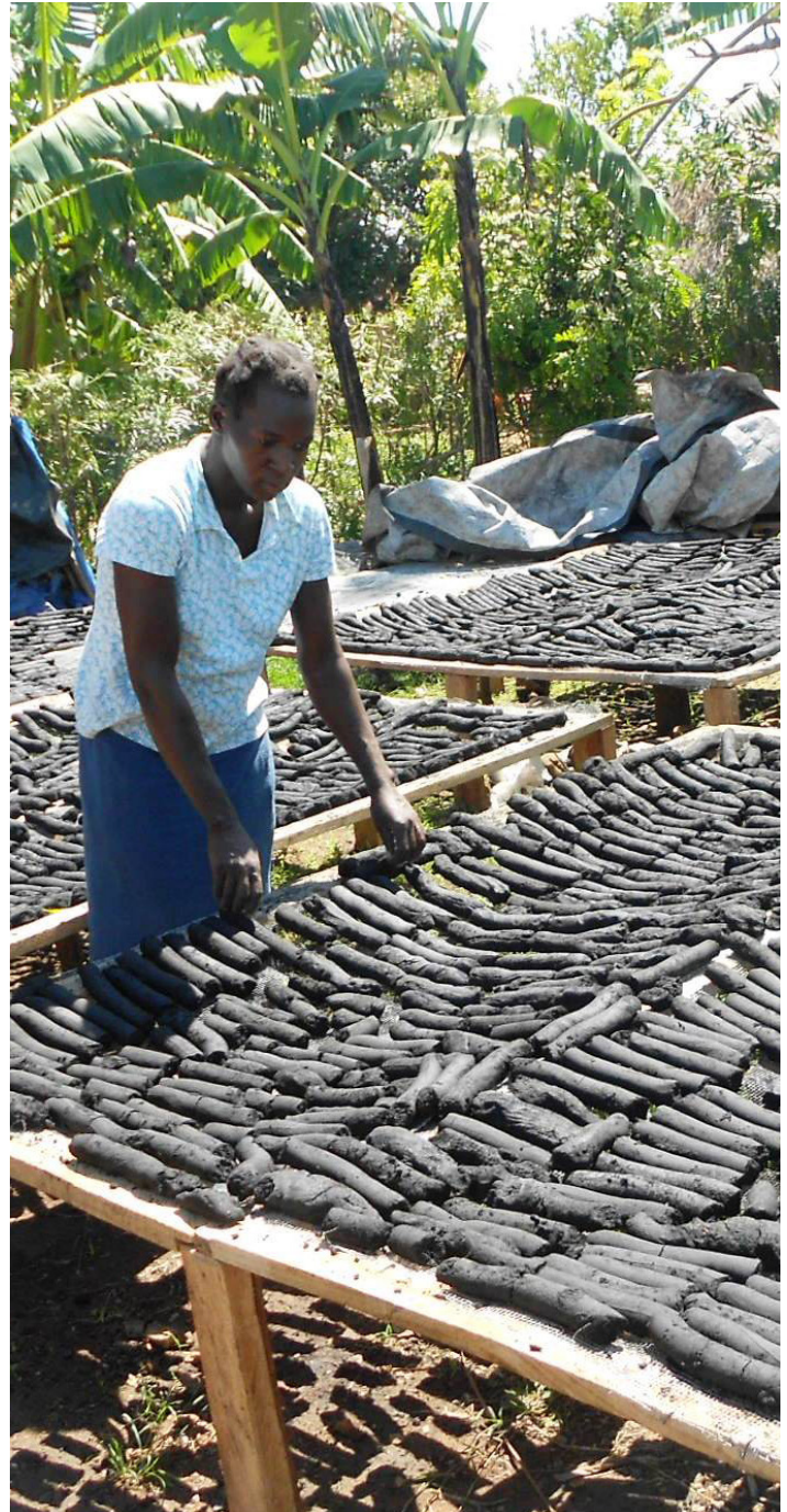
Figure 6: Drying agricultural waste briquettes at AEST.
