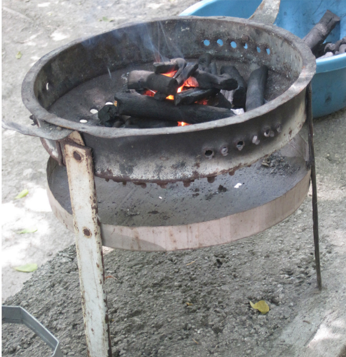
Figure 3: Un-improved charcoal burning cookstove (Metal, n.d.)
