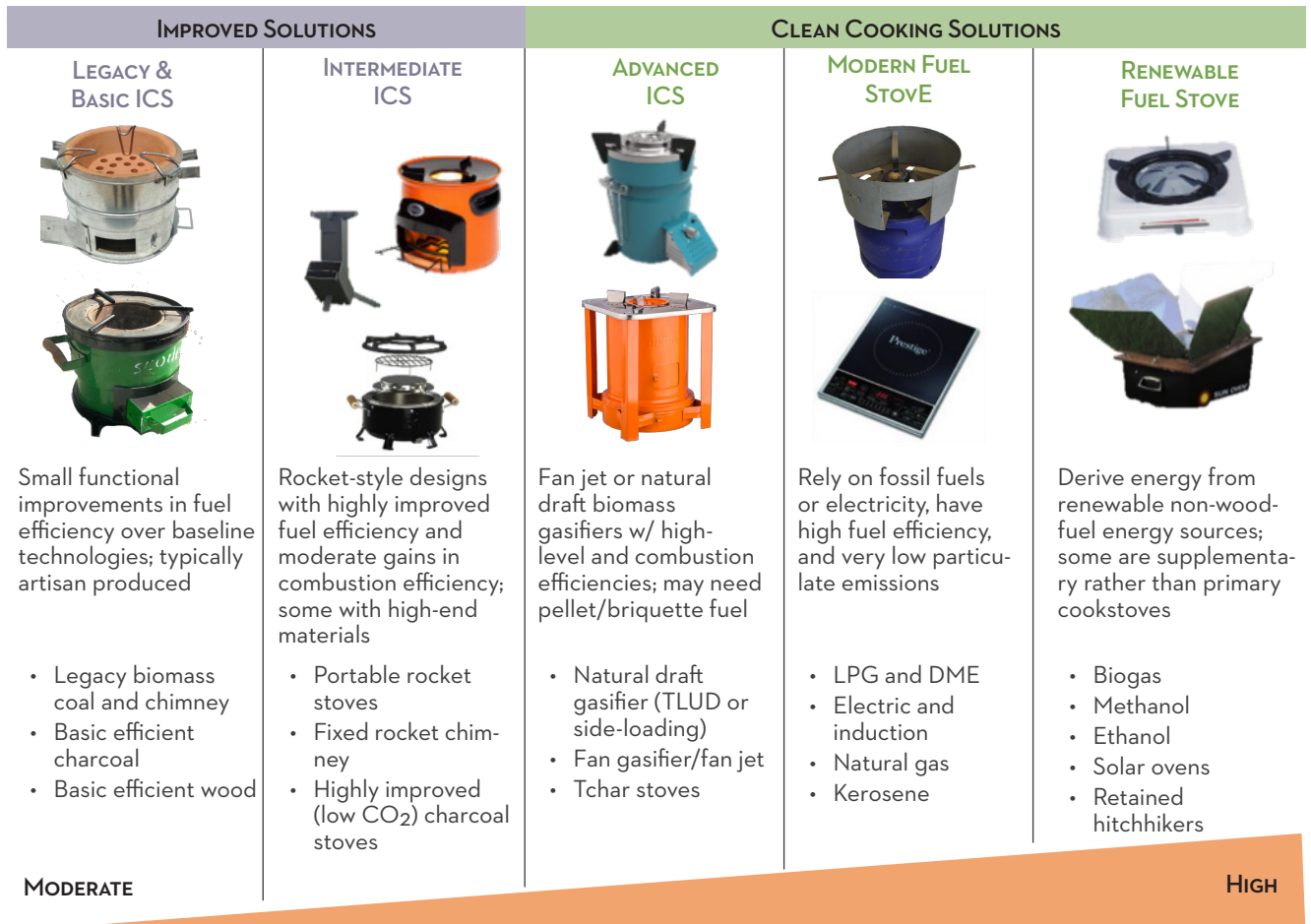
Figure 4: One framework for categorizing improved and clean cooking solutions. Adapted from the World Bank Report: The State of the Global Clean and Improved Cooking Sector (Energy Sector Management Assistance Program, 2015). The pictured stove models are for illustrative purposes only, and this report is not advocating for the use of particular brands or models of cookstoves.
