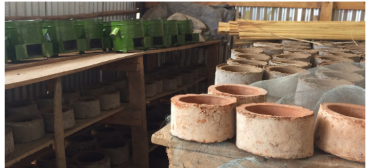
Figure 9: Completed Maaka stoves (left) and clay liners waiting for assembly (right).
