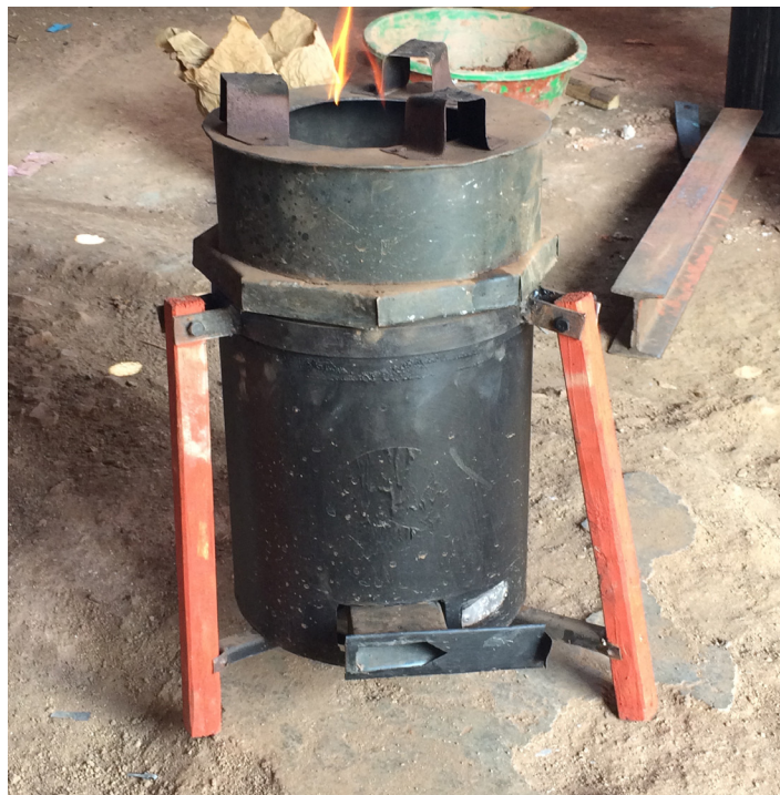
Figure 11: Awamu's top-lit updraft (TLUD) gasifier stove.
