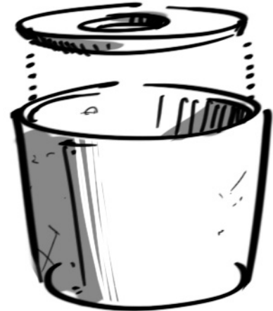
Fig 2a Press fit an endplate configuration
