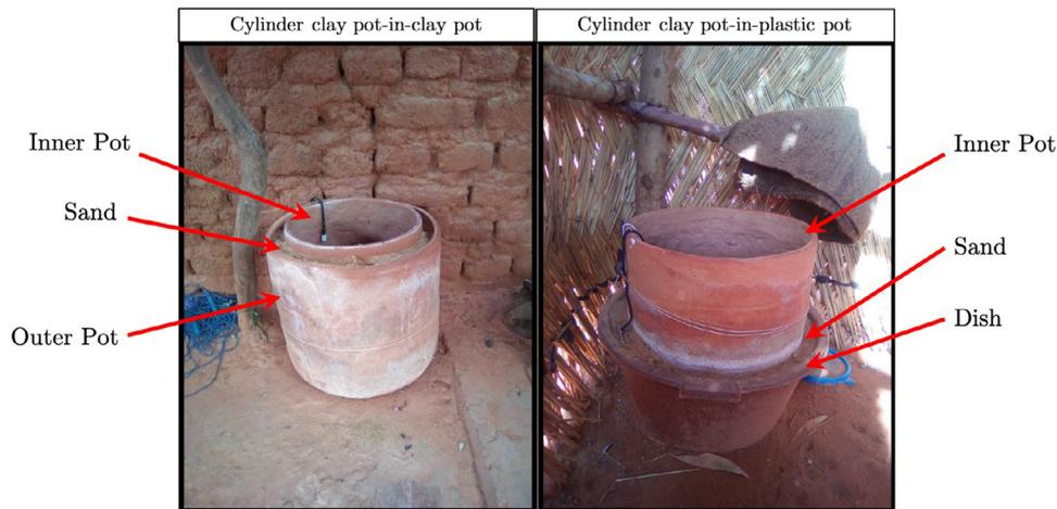
Fig. 1. Labelled clay pot in plastic dish (pot-in-dish, right) and clay pot in clay pot (pot-in-pot, left) device used from rural households in Mali (cloth not shown).
