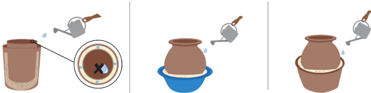
Figure 2. Schematic of three clay pot cooler devices: clay pot-in-clay pot, clay pot-in-plastic-dish, and clay pot-in-clay dish 7 .
