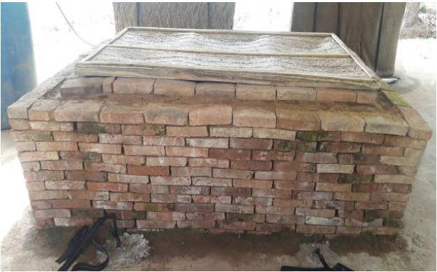
Brick ECC closed
