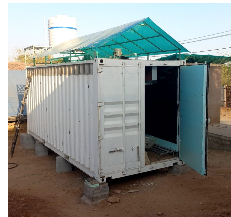
20' shipping container converted into a forced-air evaporative cooling chamber Gujarat, India.
