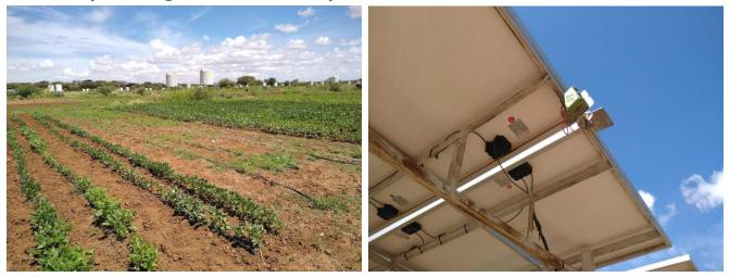
Figure 17: Drip-irrigated vegetable cultivation at Napuu 1 Drip Irrigation Scheme in Lodwar, Kenya (left), and a SweetSense gateway mounted on solar PV panels that transmits solar irrigation pump usage data to an online server via cellular or satellite data (right)
