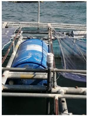
Figure 19: : Aquarech Digital thermometer installed at Nyabera Fish Cage Farm in Homa Bay
