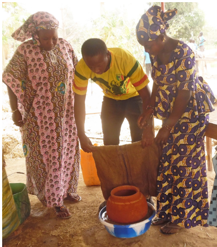
Training participants assembling a clay pot cooler at the Nyeleni Cooperative Society in Mopti, Mali.
