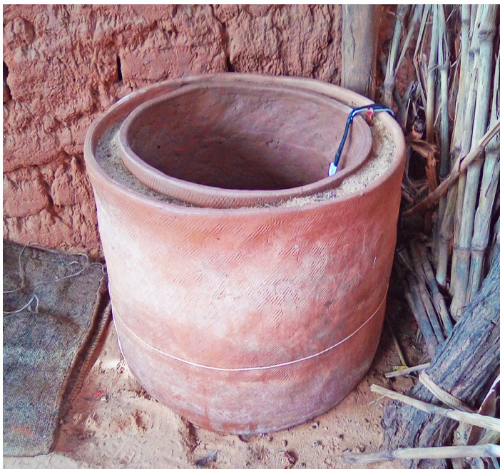
Clay pot-in-pot cooler in Bankass, Mali. Photo: Ousmane Sanogo
