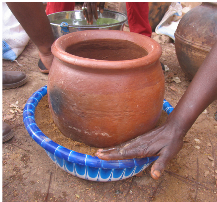
Clay pot-in-plastic dish cooler in Samanko, Mali. Photo: Ba Germain Diarra
