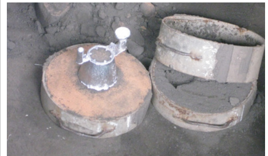
A cast corn sheller with sprues attached.
