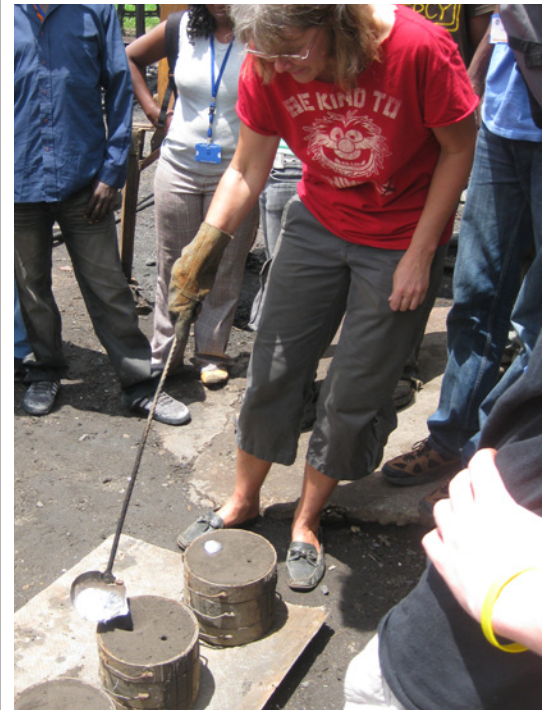
Pouring molten metal into the molds.
