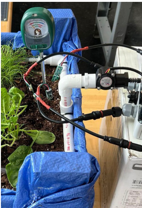
Prototype of a smart irrigation system to evaluate water use to support agricultural productivity and water conservation in the Kandahar region of Afghanistan. Photo: MIT D-Lab
