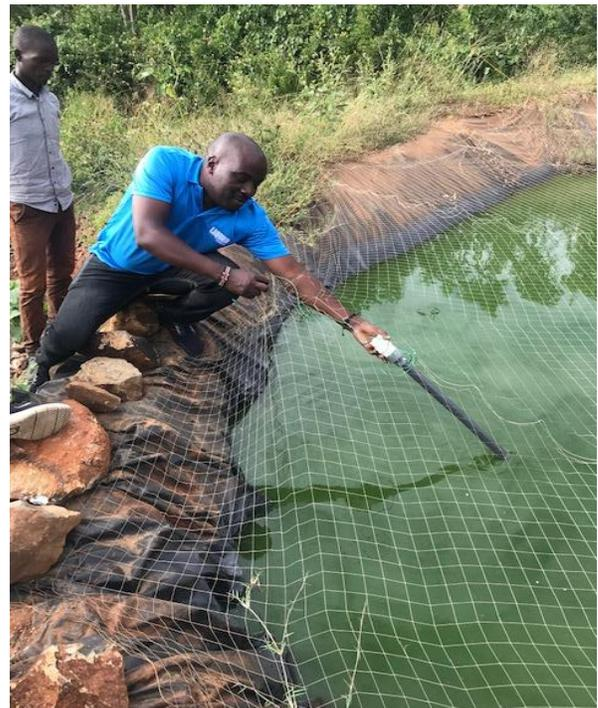
**Figure 18: Digital thermometer installation at Ramogi Institute of Advanced Technology (RIAT) Kisumu**
