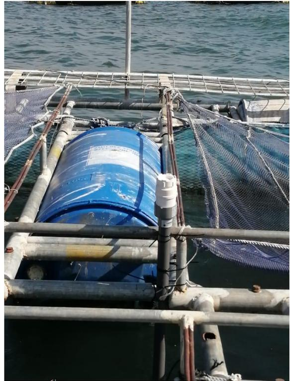
**Figure 19: : Aquarech Digital thermometer installed at Nyabera Fish Cage Farm in Homa Bay**
