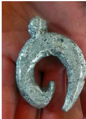
Sample of an aluminum casted maui's hook piece made by one of the participants
