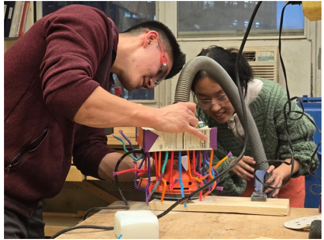
Fig. 12: A concept to use multiple straws as miniature vacuums pointed at the base of the sander
