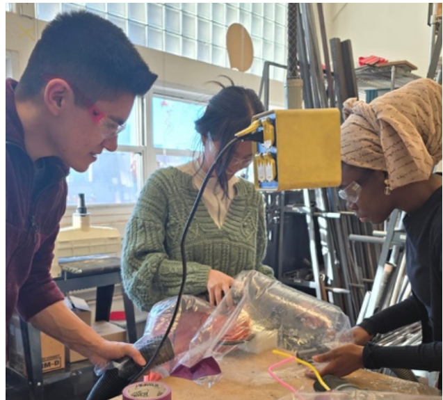
Fig. 10: A concept for a bag over the sanding location being tested
