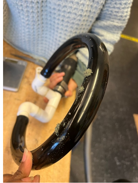
Fig. 17: Dust clogging small holes in the vacuum tube
