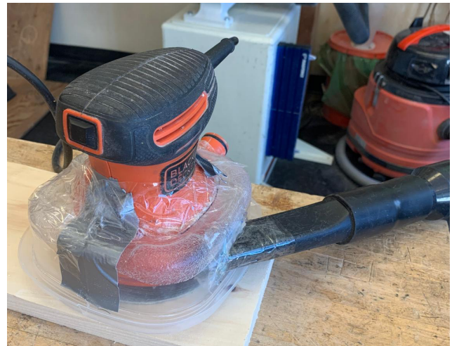
Fig. 13: A vacuum attached to a shield around the sander
