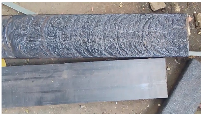
Fig. 5: Top plank - just extruded; bottom plank – after refinement and sanding
